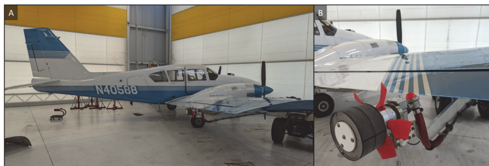
Figure 1. (A) Piper PA-23-250 Aztec airplane (Reg# 203DM) used by the Salt Lake City Mosquito Abatement District, Utah, USA, for aerial ULV adulticide applications. (B) Equipped with Micronair AU4000 rotary atomizers.
